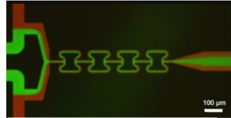
Not mixed well Flow rate: 1 \mu\text{L/s}
