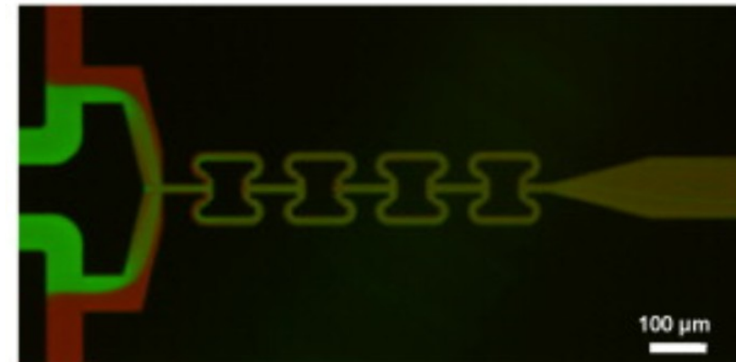
Very well mixed Flow rate: 6 \mu\text{L/s}
