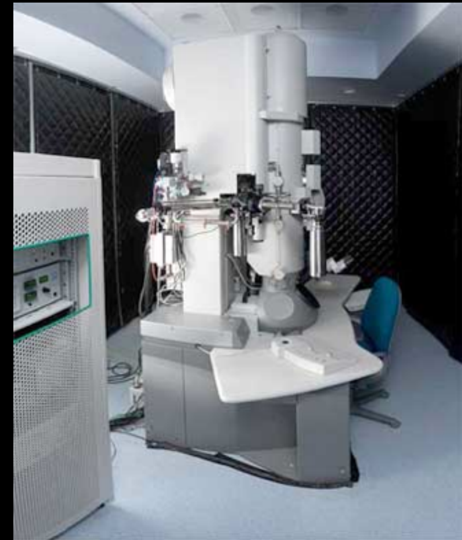
FEI Polara @ 300 keV Gatan Quantum energy filter Gatan K2 summit detector
