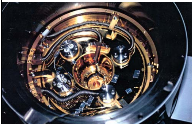
Helium stage for high resolution electron microscopy
